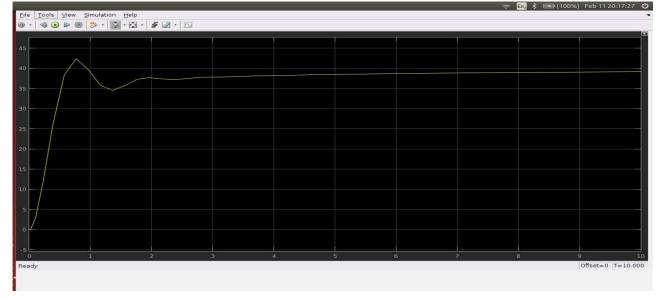
By setting up proper values for Kp,Ti,Td etc the temperature and moisture level values are controlled which helps in achieving our objective of automation and real time monitoring. PID control gives best results and helps in achieving our goal of precise automation by modeling and controlling both input and output parameters.
